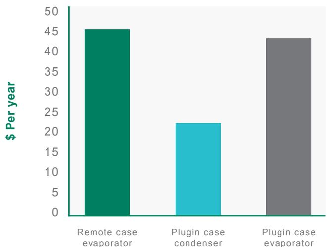
Based on \$0.11/kWh and 200/28 fan at 1550 RPM
